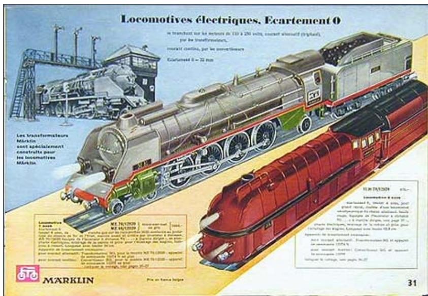
The model, constructed in tinplated steel, and finished in a bold maroon color, is notable in that the wheels are hardly visible! This was truly a well-shrouded locomotive! Marklin saved some money by eliminating the valve motion (but it has main & side rods)
