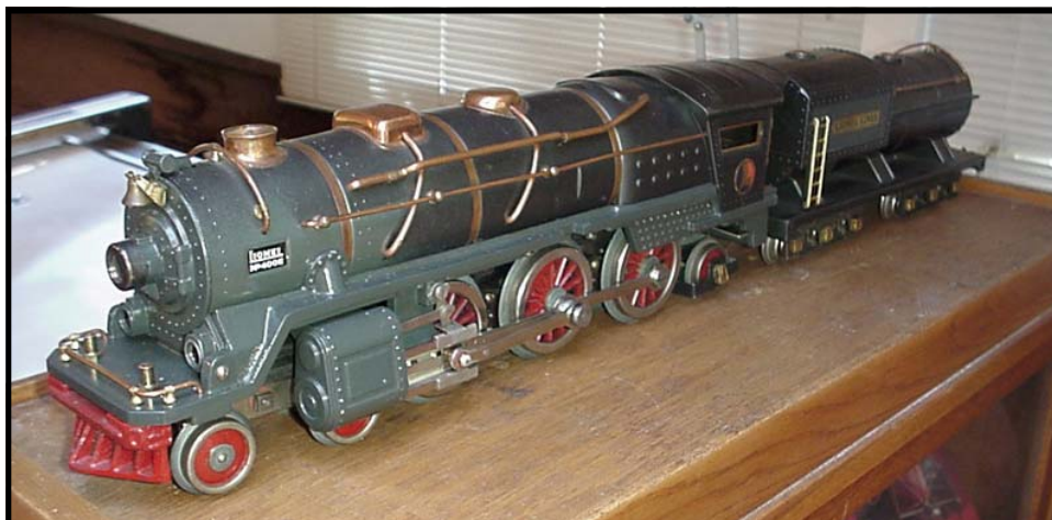
Nor Cal member Chuck Schaeffer's Lionel Standard Gauge #400E, normally a 4-4-4, converted to a 4-6-2, and altered to run on Carlisle and Finch 2-inch gauge track. This involved changes to the boiler and frame, as well as the motor.
