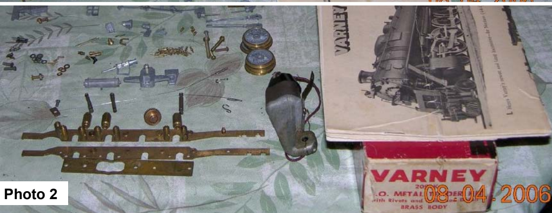
Photo 2: shows the parts needed to make this kit up as a “Super” Northern: a two-piece brass frame with spacers, for sprung drivers, and a V2 motor.
