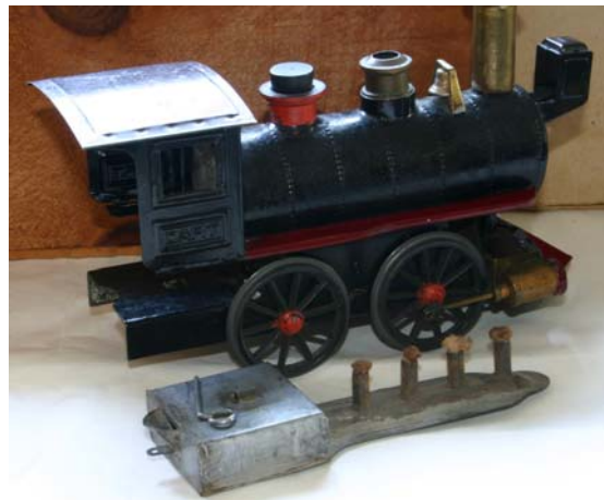
Photo 8—National Playthings (?) loco with the "late" type four wick burner unit removed
