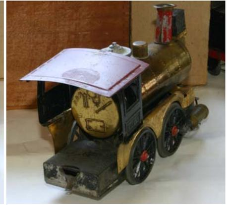
**Photo 3—showing the brass boiler backhead**
